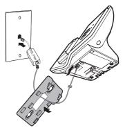
2 Align the holes on the bracket with the standard wall plate and slide the bracket down until it clicks securely in place.
